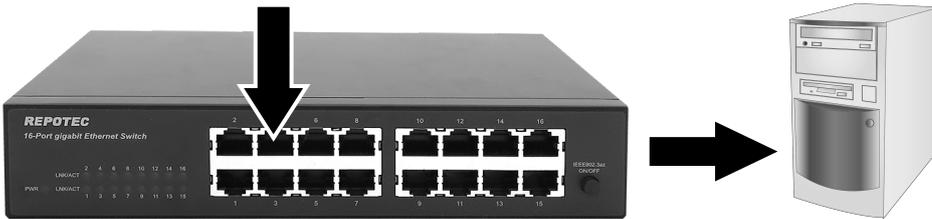
3. Move the power switch to the On position.
