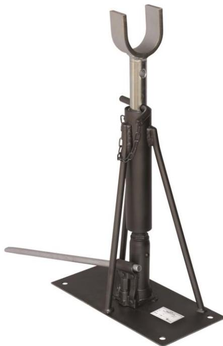
Hydraulic lifting drum stand made of galvanized steel. Composed by a steel structure electro-welded on a flat ground base, a pivot holding head fixed on support shaft with 4 adjustable position, made of galvanized steel, 360° rotating and a support shaft lock pin with chain. Adjustable height by means of hand operated hydraulic piston
