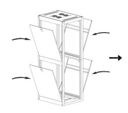
When assembling the side panels, it is necessary to lock the panels and remove the keys in case of falling down!
