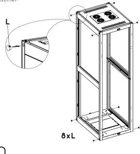
When assemble the whole frame, the plastic cover(L) should be removed.
