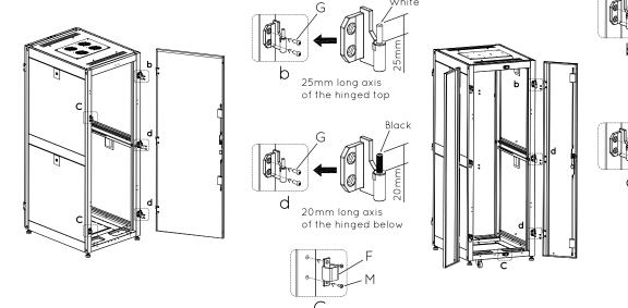
25mm long axis of the hinged top d 20mm long axis of the hinged below
