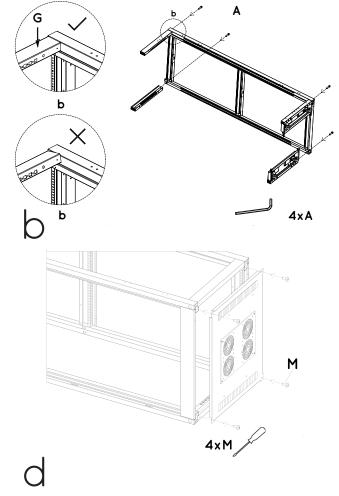
For the cabinet over 800 depth, the fans should be assembled closed to the rear door.
