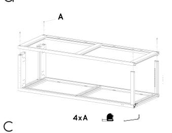
After assembling, if the diagonal framework is more than 4mm, it is required to loosen the bolts and then reassembled;
