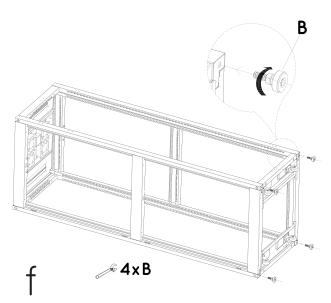
After assembling, the M12 feet should be under (shorter than) the castors in case of breaking when set up the cabinet!
