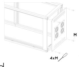
For the cabinet over 800 depth, the fans should be assembled closed to the rear door.
