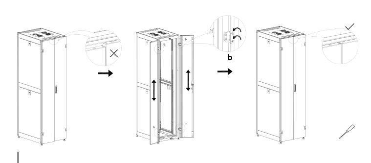
Doors can be adjusted by loosening hinge screws, moving the door and retighten.
