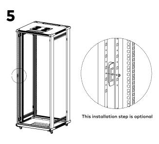
This installation step is optional. With 2 x bolt M5\*10 (A) fix this accessory to the frame;
