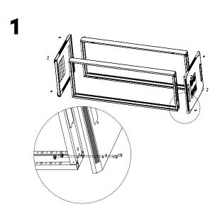
In this first step you will need the top cover (5), the bottom plate (8) and  $2 \times$  frame (6). Put the two parts of frame ready to assemble this part like picture with 16 x bolt M8\*12 (C) and 16 x flange nut M8 (D);
