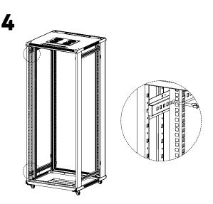
With the cabinet in the vertical, assemble the mounting angle (4) with 16 x bolt M6\*12 (B) in the horizontal sides of the cabinet;
