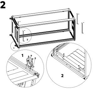
With the cable entry panel (9) and with the castors (10), assemble in the bottom plate with  $24 \times 10^{10}$  (A);
