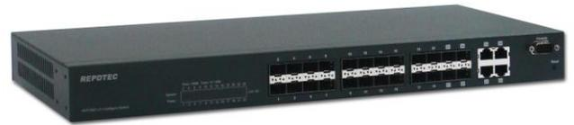
RP-GS2024I is a cost efficient and high-performance L2+ Ethernet management switch - 20-port (100/1G) SFP+ 4-Port SFP/RJ45 combo are supported. This switch supports remote management by SNMP, Http and Telnet interfaces, and local management by console interface. RP-GS2024I supports lots of L2 switch management functions, e.g. 802.1Q VLAN, 802.1x Security, Rate Control, Port Configuration, Port Mirroring, Port Statistics, QoS functions, ... etc.
